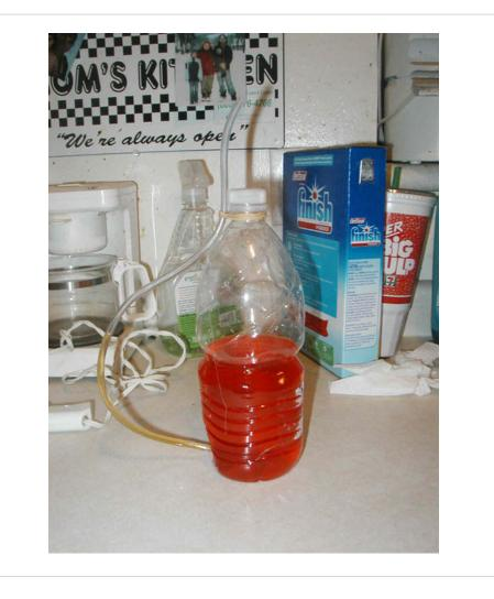
This is an easy project and would make a great science experiment. Using a vacuum inside a plastic bottle with water in it, you can observe the changing air pressure with this simple barometer. Please note, this type of barometer only allows you to see if the air pressure is high or low.
