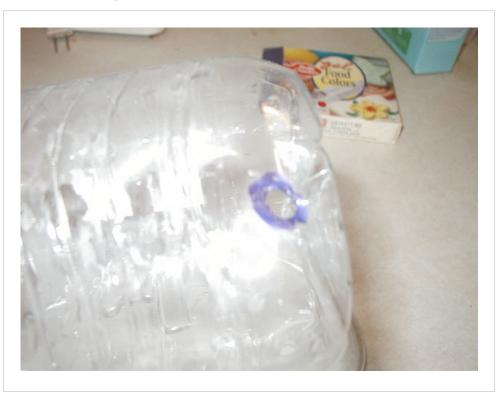
Using the nail, make a hole in the bottle slightly smaller then the outside diameter of the tubing at the base of the bottle. This is to ensure you get a tight seal. I actually heated the nail using my stove top to make this easier to do, and the heated nail allows for more accuracy.
