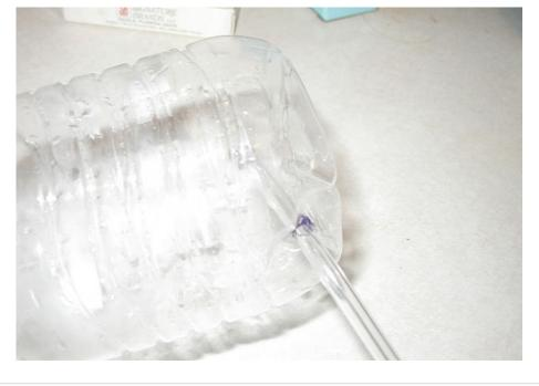
Insert the tubing until the tip is half way into the bottle, and should be resting on the bottom of the bottle. You may need the help of the cooled nail to insert the tubing. Remember, it must be a tight fit.
