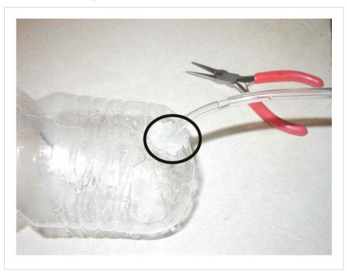
Fill the bottle with enough water to come up about an inch on the bottle. If it leaks, dump the water out and apply a good size bead of low-heat glue around the tubing on the bottle. When the glue has cooled slightly, use your finger to push the glue into the area surrounding the tube to make a water-tight seal. Let cool, and check for leaks again. If still leaking, apply more glue.
